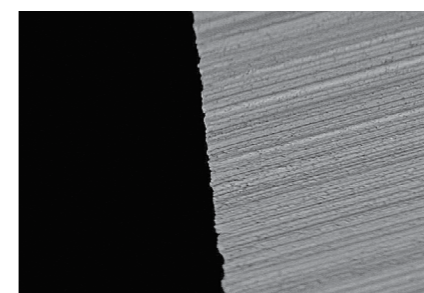
5000x zoom of an unmachined cutting edge
