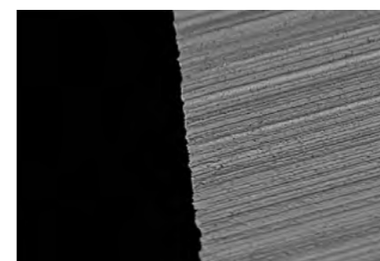
5000x zoom of an unmachined cutting edge
